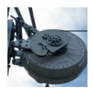
By means of a support cable, TENSOREX C+ exerts a constant tension on the contact wire, regardless of any changes in length due to temperature. The special spiral spring is firmly connected to two cams on the same shaft.
